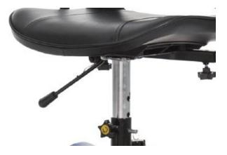
**8.** Use the lever to release the seat and turn it so that it faces the front of the handlebars. Then use the lever to lock the seat in position.
