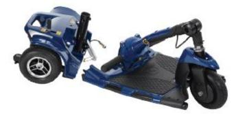
7. Lift the part where the two parts are connected and release them from the hooks.
