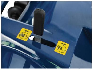
**WARNING**: Never switch the scooter to manual mode unless you have the assistance of another person. Do not switch the scooter to manual mode on hills or inclines. Failure to follow these instructions may result in personal injury or property damage.
