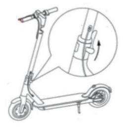
2. Attach the grips to the handlebars, be careful not to pinch the cables.
