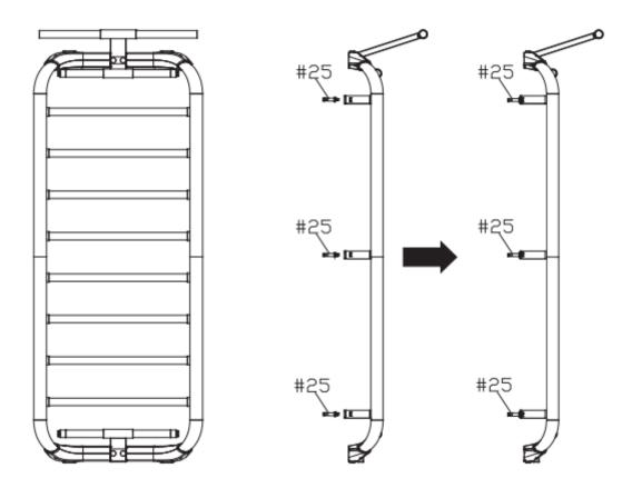
Attach the wall bars to the prepared holes in the wall using a dowel and expansion screws (M8\*80 mm).
