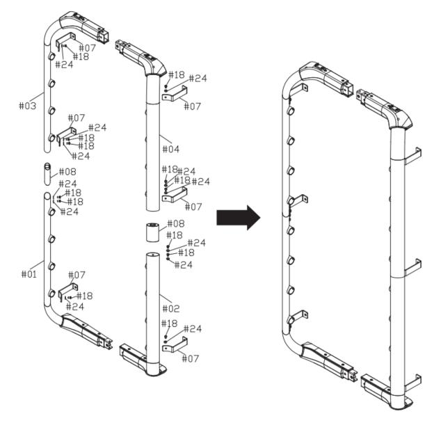
Attach the connecting frame (08) to the lower frame (01) using screws (18), washers (24) and a wrench (28).
