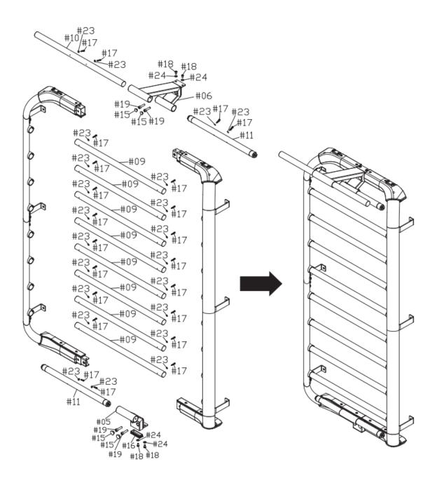
Attach the bar (11) to the step holder (05) using screws (17), washers (23) and cover (16).
