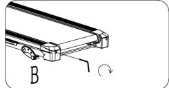
Over time, the running belt (20) will loosen. To tighten the belt, turn both the left & right-side adjustment bolts one full turn clockwise. Check the tension of the belt. Continue this process until belt is at the correct tension. Make sure to adjust both sides equally to ensure even belt alignment. Refer to image C.
