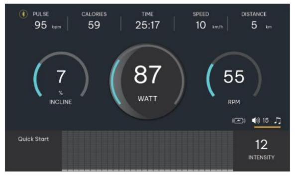
**PULSE:** If you wear the chest belt or hold the pulse sensors on the handles, the pulse rate will be displayed
