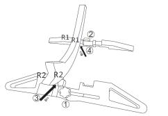
Loosen the hand knobs (1 and 2). Pull the rack apart so you can see the screw holes. Attach the sides as marked R1 to R1, R2 to R2.
