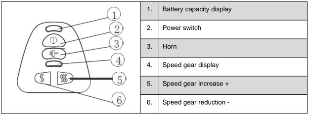
The on / off button is used to switch the truck on / off. In emergency situations, it can be used to switch off the wheelchair immediately.
