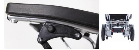
Release the rear beam, release the U buckle.
